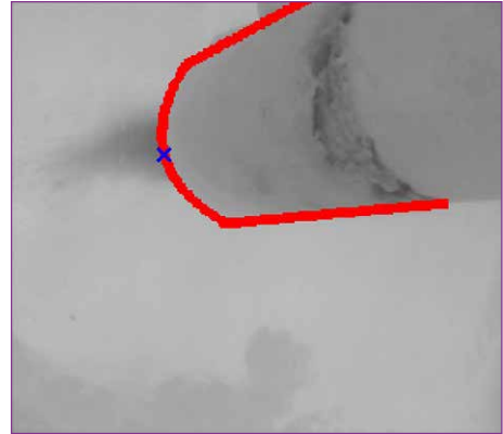
Figure 5: Template matching for burner tip detection
