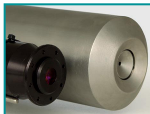
Figure 4: NIR camera and combustion chamber probe
